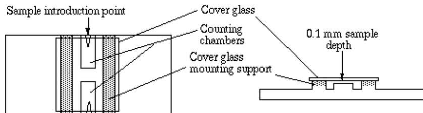
To prepare the hemacytometer, the mirror-like polished surface is carefully cleaned with lens paper and ethanol. The coverslips (which is thicker than those for conventional microscopy) should also be cleaned. The coverslip is placed over the counting surface prior to adding the cell suspension.
